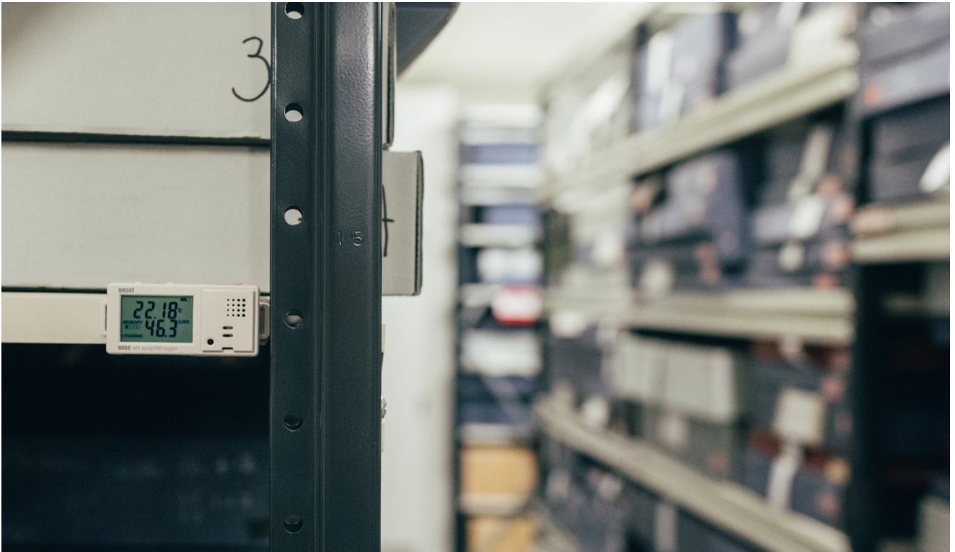
Temperature and Relative Humidity logger in a collection store room. Image: Tiny Empire Collective
