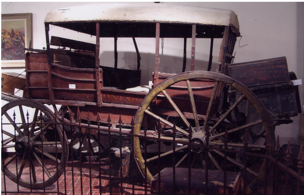
This stage coach was owned by Heber C. Kimball's Freight Company. Careful inspection shows it to be at grave risk. The axles are very weak and about to fail. In addition, the leather is cracked and the wood is split. This coach needs to be conserved and stabilized to prevent collapse. Pioneer Memorial Museum
